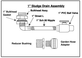
permanently if you wish. It will not impede the normal function of the sludge drain. <u>Caution: You must set your control</u> <u>head to the Backwash or Rinse position before turning on the water, otherwise damage may result. Most household</u> <u>water pressures are between 60-80 psi. This is too much pressure for the filter tank. The Backwash or Rinse position</u> will vent all of the hose pressure to the waste line which will cause no harm at all.
