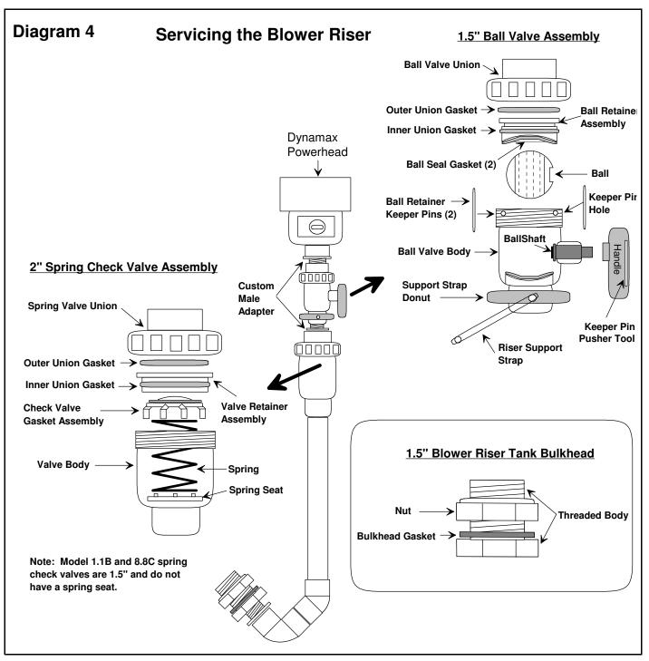
Servicing The Blower Riser Components (Visual Reference Diagram 4)
